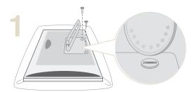
Cover the floor with soft cloth or a cushion. Place the wireless TV face down and unfold the TV's stand. Unscrew the screws at both sides as shown in the figure. You can use a coin or a screwdriver to loosen the screws.
